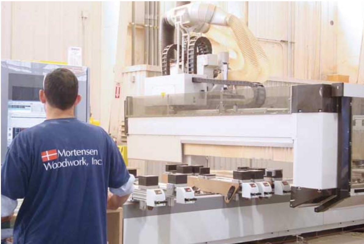
The Busellato five-axis CNC machining center has pods for horizontal and edge machining of panels.
