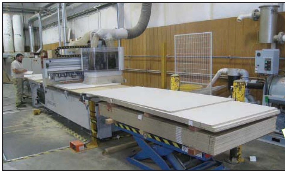
The Linear Flow system used on a Busellato Optima router at Custom Source Woodworking. Fully nested casework or paneling are processed on this machine.
