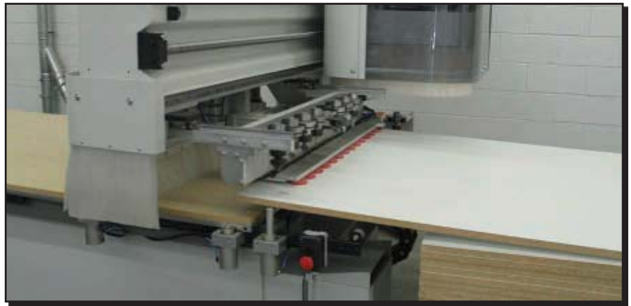
A closer look at the Linear Flow system pulling a panel into the cutting area in the demonstration area at Delmac headquarters in Greensboro, N.C..
