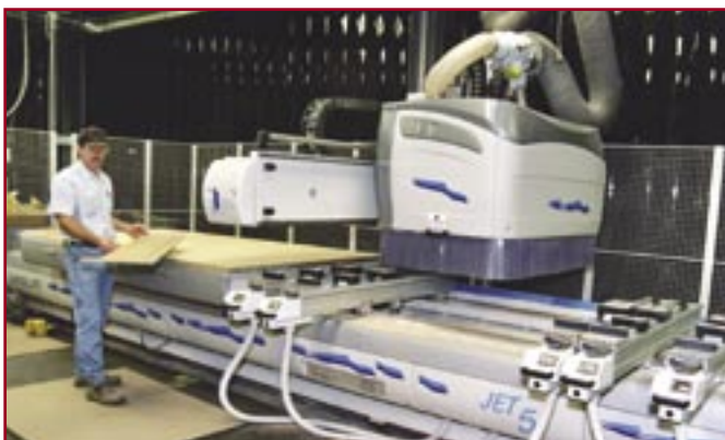
Burger Boat added a Busellato Jet machining center to its millwork department. The unit produces complex parts for the custom interiors.
