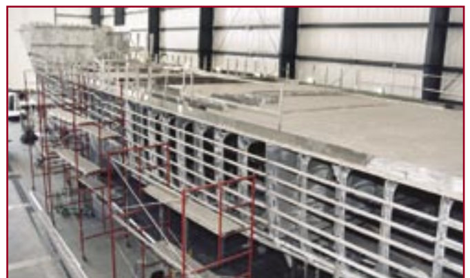
The super structures of the yachts produced at Burger Boat are made of 5,086 aluminum alloy.
