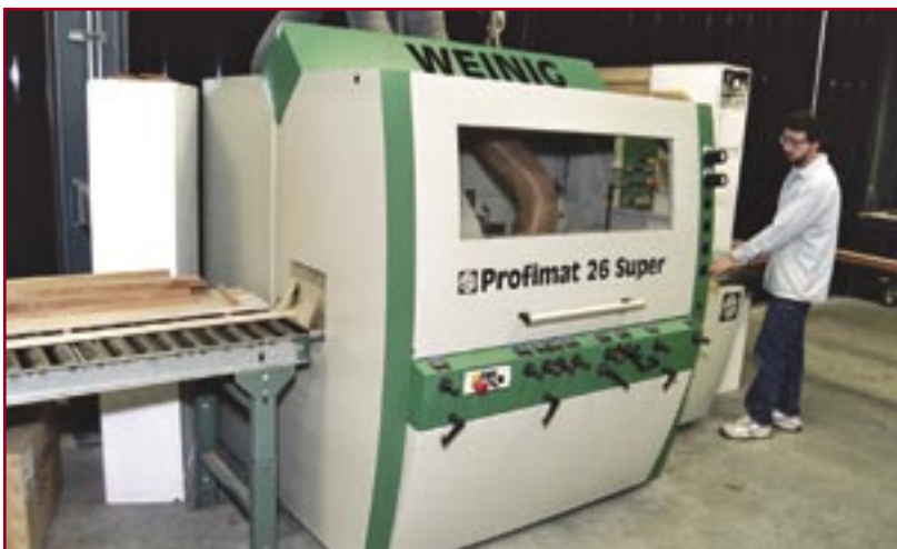
Mouldings and other profiles are produced on a Weing Profimat 26 Super moulder in the millwork department.
