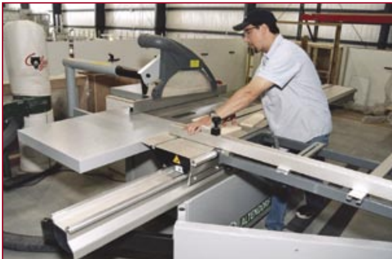
Panel cutting is handled by an Altendorf sliding table saw in the upper level of the millwork shop.
