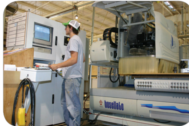
Keystone Millwork depends on its Busellato JET 400Z RT CNC router to provide the flexibility needed to handle the variety of jobs it takes on.
