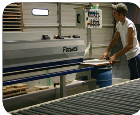
Bob Kraus, president of Keystone Millwork, CNC equipment, such as this Fraval RX-5 edgebander, has brought increased efficiency and accuracy to his company's projects.
