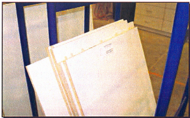
All parts are barcoded and stacked on carts for moving between stations in the shop. Special efforts are made to keep parts together in convenient assembly order throughout the process.
