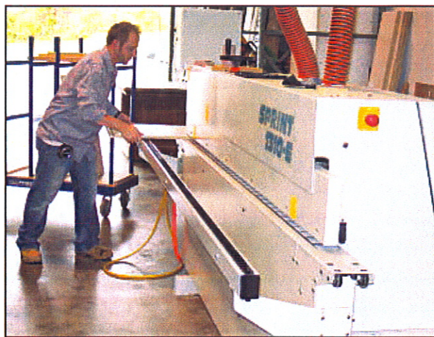
After doweling, parts needing edgebanding are processed on the Holz-Her Sprint 1310-E edgebander.
