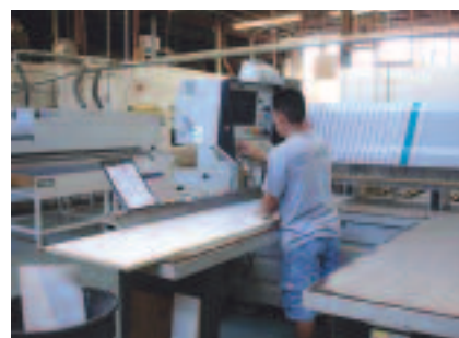
Melamine boards are cut to size on the shops' Meyer PS9 10-foot beam saw.
