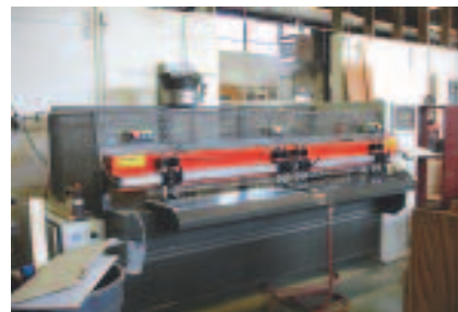
Panels are bored on this Gannomat 271 drilling machine.
