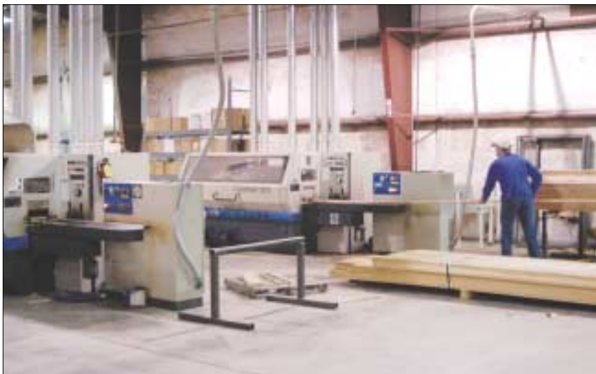
Two Weing Unimat 23E moulders handle all the milling for the company's door, window and molding lines.
