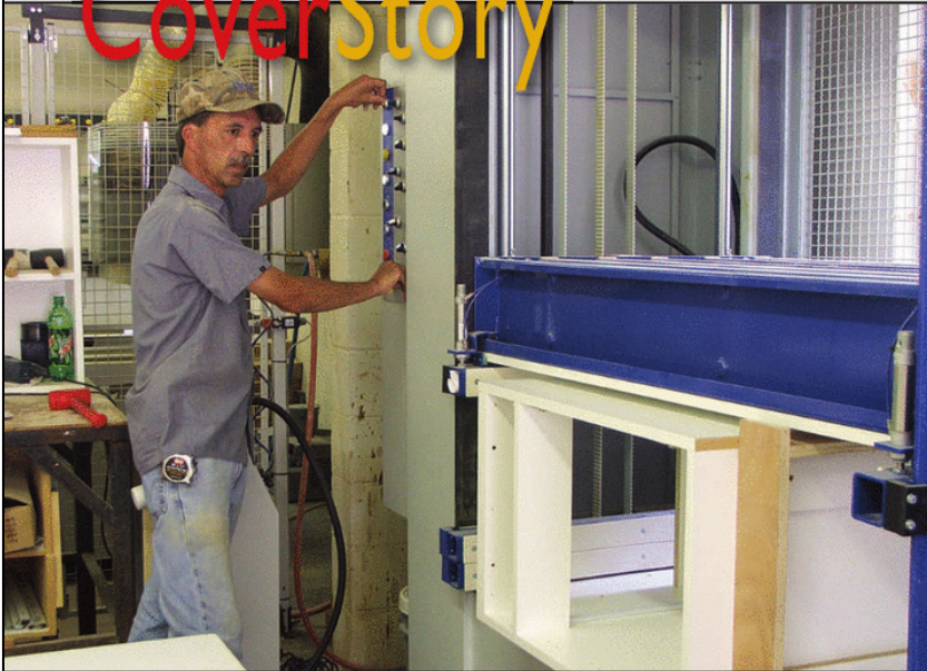
Fast and square — A key part of the move to automation at the James Cabinet Shop is this Bonacin Closer 30-inch case clamp, left, which speeds box assembly and glue-up.
