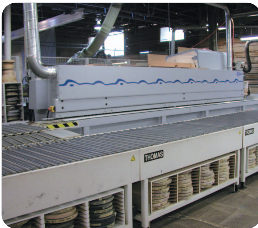
Interscapes purchased the largest Brandt edgebander it could find at the time, the KDN-980 2C Optimat, to handle the edgebanding requirements of two production lines.
