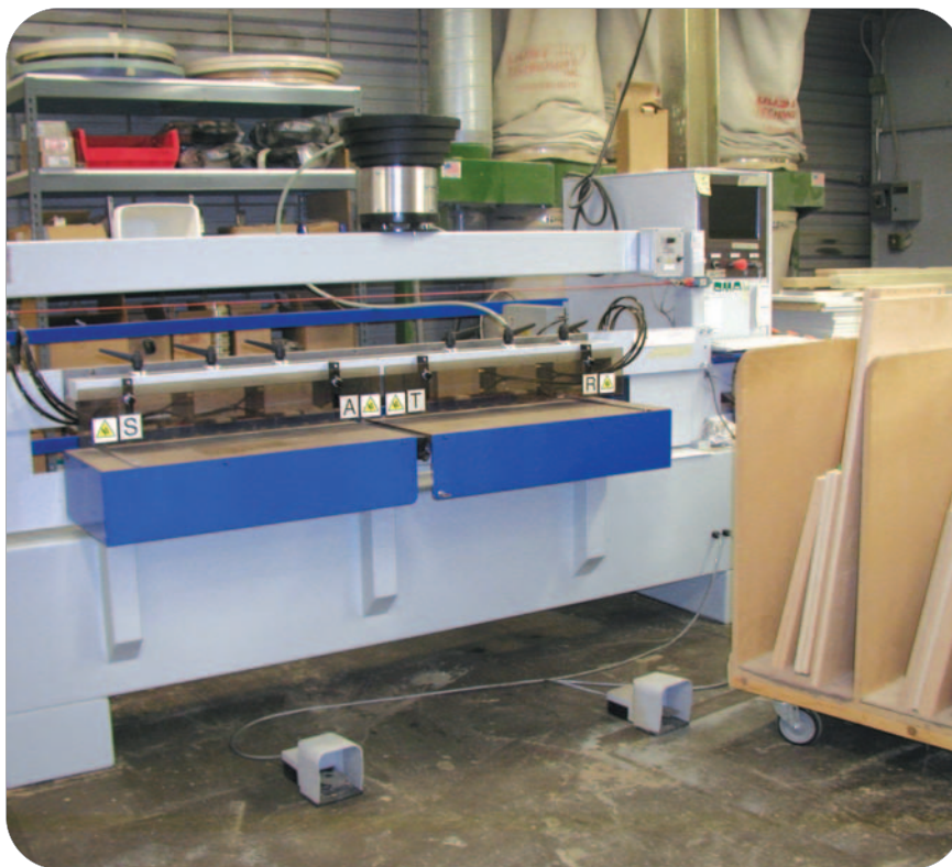
To speed production, Interscapes moved the horizontal boring functions from the point-to-point machining center to its new OMAL horizontal bore, glue and dowel insertion machine.
