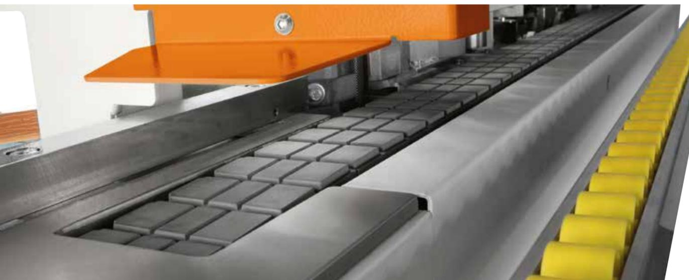
Linear and perfect feed thanks to feeding chain track with high grip rubber coated pads and sliding on industrial chain. High resistance to lateral loads thanks to special guides with one circular section and one flat section. Feed speed until 22 m/min available on request.
