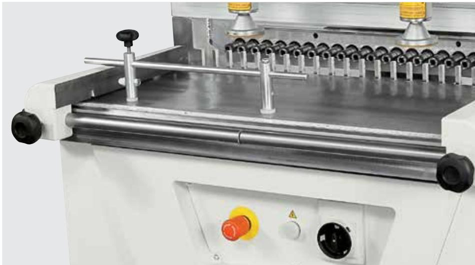
Reference compass for positioning the guides in specular mode (standard).
