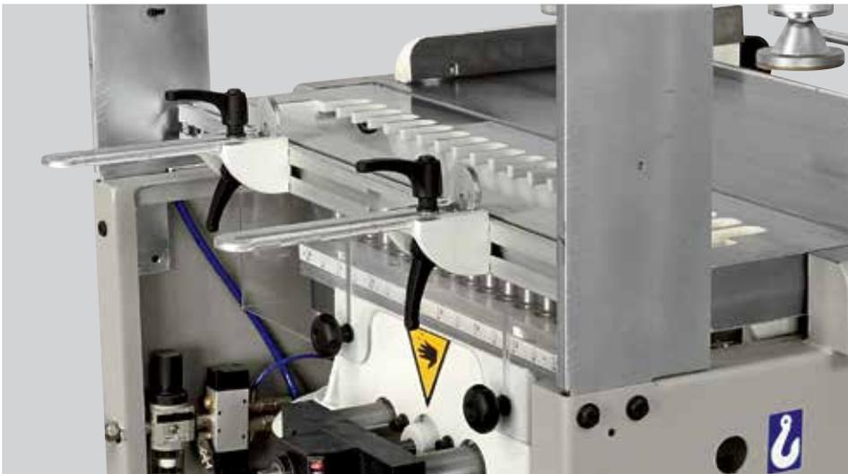
The machine is equipped with 2 adjustable depth stops as standard which can be used during vertical boring as a panel support reference
