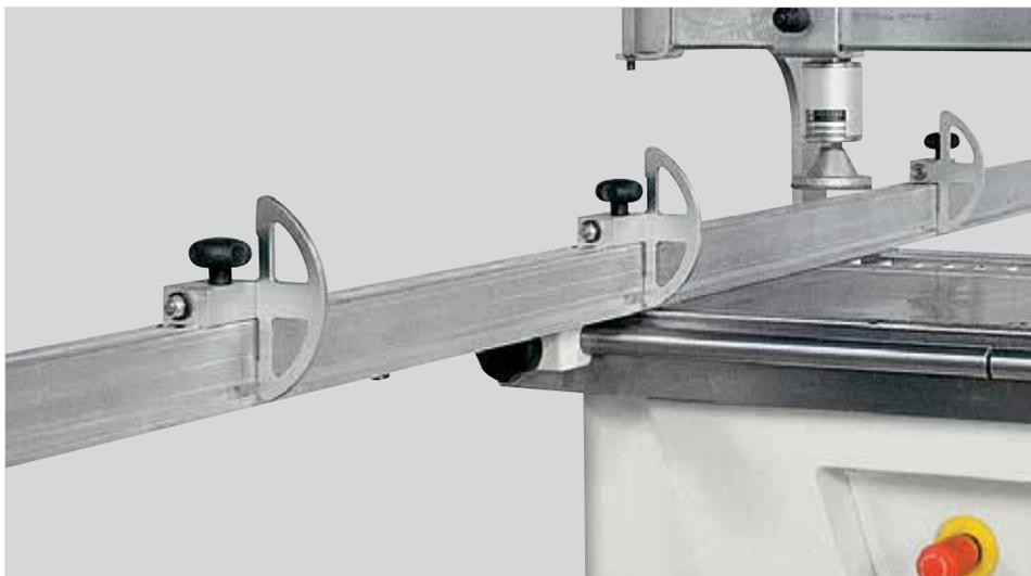
Lateral fence L=3000 mm, used for multiple linear boring.
