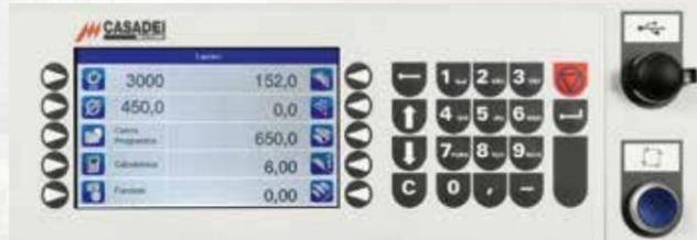
Numeric Control, standard on all "A" versions with 7" LCD colour display 16/9 format. Possibility to control all axis of the machine, alphanumeric keypad, storage capacity up to 300 working programs, control of the spindle rotation speed (if the machine is equipped with inverter), USB port to load working parameters.
