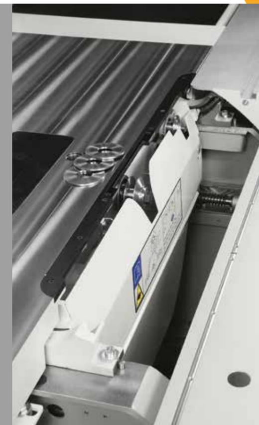
Overhead saw guard with built-in dust collection port. Standard for all CE and USA/Canada versions.
