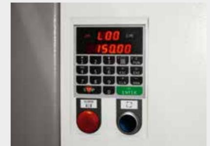
The thickener table electronic positioner, available on request, enables fast and precise worktable positionings. With calculator included.
