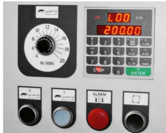
The thicknesser table electronic positioner, available on request, enables fast and precise worktable positionings.
