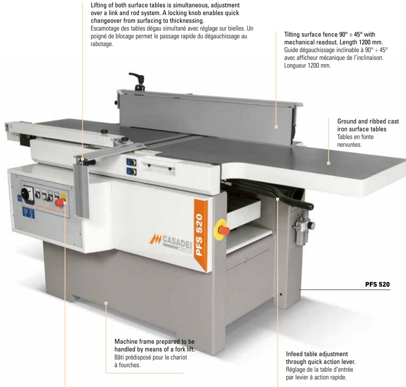
Lifting of both surface tables is simultaneous, adjustment over a link and rod system. A locking knob enables quick changeover from surfacing to thicknessing.
