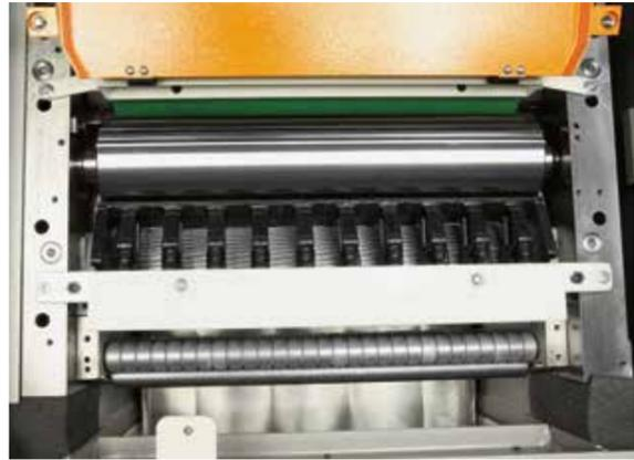
Planer unit with infeed anti kick-back fingers and segmented chipbreakers, serrated steel infeed roller with spiral teeth and rubber coated outfeed roller. Feed rollers are interchangeable.
