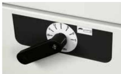
PS 520: 4 feed speeds (5/8/12/18 m/min) through mechanical selector.
