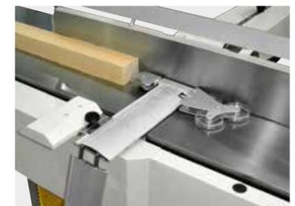
The "TX MATIC" cutterhead protection with automatic raise & fall, available on request, raises the cutterhead safety cover only during material feed. In this way the cutterhead is covered at all times, for enhanced safety.
