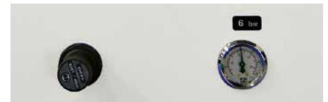
The PS 630 can be equipped, upon request, with pneumatic adjustment of the top feed rollers pressure from the front control panel rather than mechanical. The pneumatic pressure guarantees the same pressure with any stock removal.
