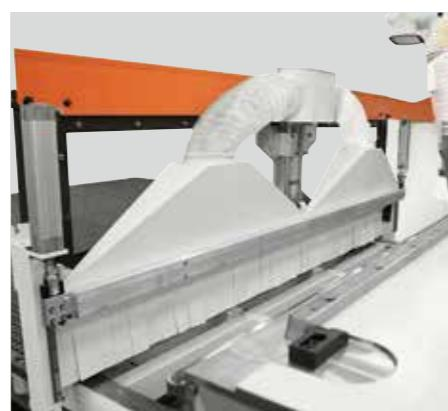
Unloading device w/ integrated suction system (optional)
