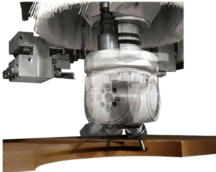
0 + 360 unit: flexibility without limits. Unit with digital control managed by numerical control for positioning at 360° of the angular aggregates. (optional)
