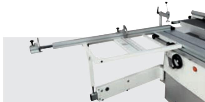
The very strong, large sized, squaring frame is supported by a strong telescopic arm. The squaring frame is tiltable  $\pm 45^\circ$  and is equipped with 2 retractable stops and eccentric clamping.
