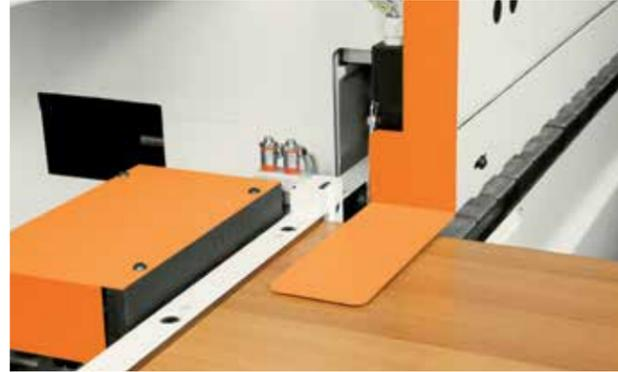
Device for spacing the panels at the entry to optimize the spacing between the panels according to working units. Standard for Flexa 607 and XE versions.
