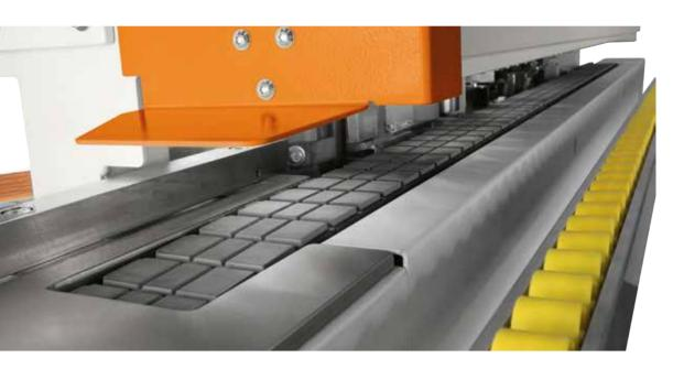
Linear and perfect feed thanks to feeding chain track with high grip rubber coated pads and sliding on industrial chain. High resistance to lateral loads thanks to special guides with one circular section and one flat section.
