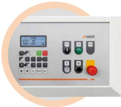
The machine is equipped with the Mega 120 control unit placed in ergonomic position and with on/off buttons for the different working units. Control unit MEGA 150 TS with 7" touch screen available on request.
