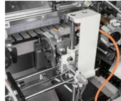
**Cutting unit.** The unit is equipped with 1 high frequency motor for the frontal and rear cut of the edge at 90°.
