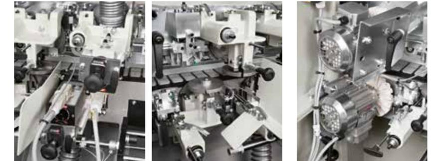
**Trimming unit.** The trimming unit is equipped with 2 high frequency motors, each one with frontal and rear pad copiers for perfect tools positioning.
