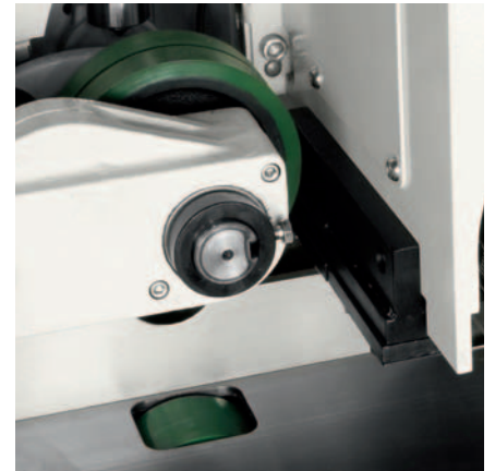
Rubber coated bed roller, after the top horizontal spindle
