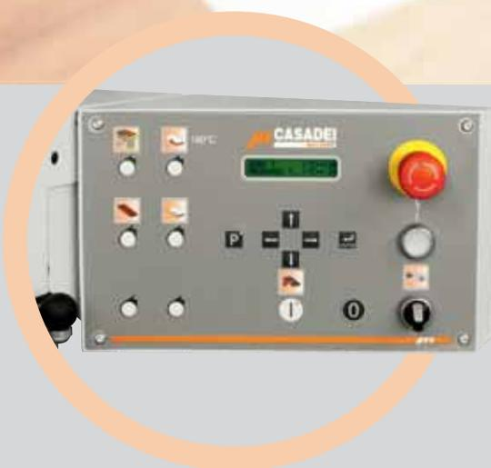
Control panel positioned at the machine's infeed in an ergonomical position. The whole machine and all working units present are controlled by PLC.
