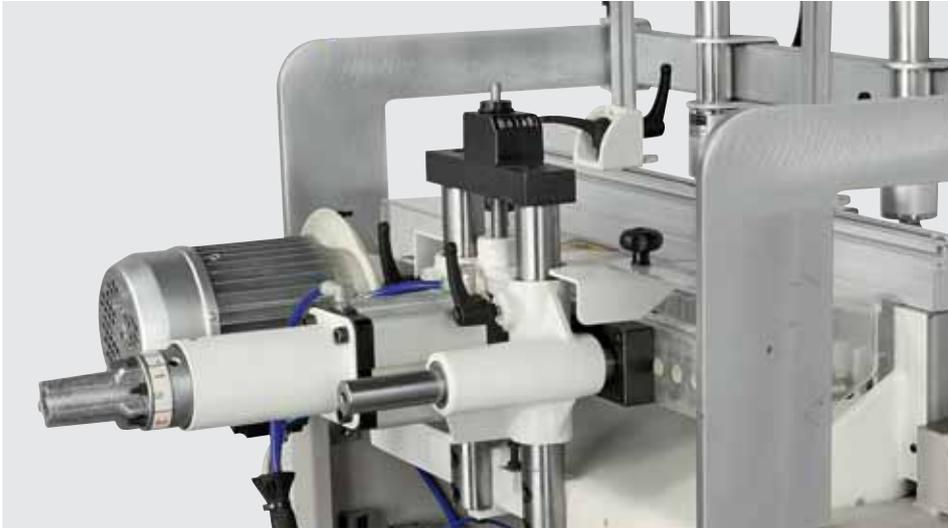
The boring head can be adjusted both in height and depth. Depth adjustment is by means of a revolving turret whilst micrometric height adjustment with decimal numerical indicator is by a handwheel.
