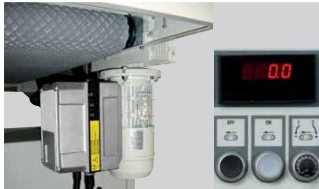
**Feed conveyor speed adjustment**
