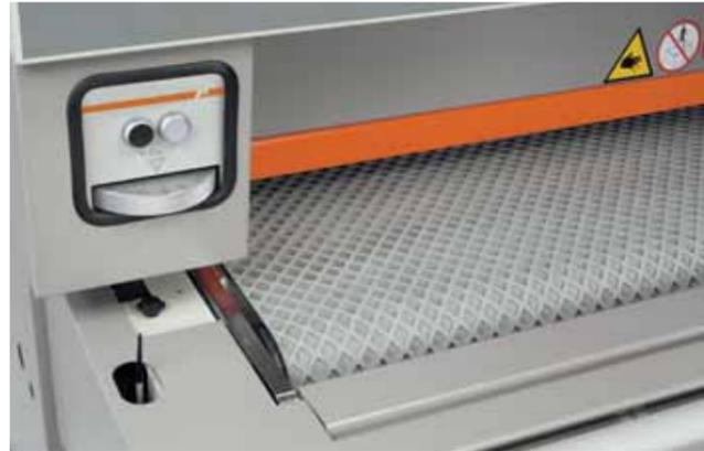
**Electronic device for worktable positioning**
