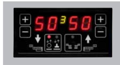
FOX 500 KRT. This control unit synchronises the lowering and raising of the platen to any feed speed rating of the conveyor. Available, on request, for all machines of the range.
