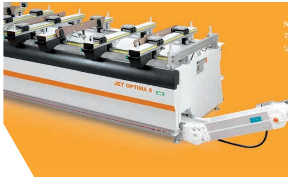
Belt conveyor for chip evacuation for maximum cleaning
