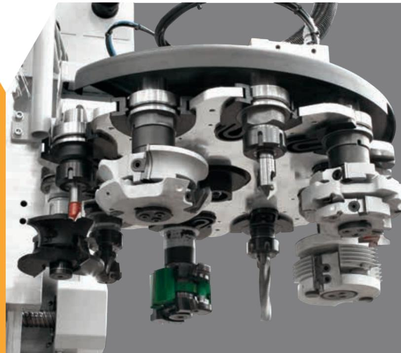
The JET OPTIMA P and S machines can be equipped with a rotary tool changer (BT) and a 16/24-position rear tool changer. The high configurability of the working units together with a large number of tools allow various solutions for machining solid wood and furniture parts.
