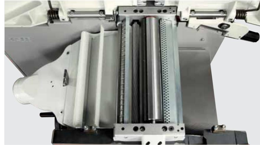
Steel cutterblock with 3 knives. The infeed steel roller has helical gearing to facilitate introduction of parts. Adjustable feed roller pressure.
