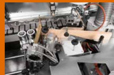
**Magazine for strip edging.** The magazine for strip edging allows to load solid edges up to 5 mm. Available on request.
