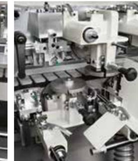
**Edge scraping unit.** The highly rigid structure allows an excellent finish PVC/ABS edges. The high machining accuracy is ensured by front and vertical pads copiers. Available on request.
