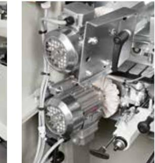
**Brushing unit.** The unit is equipped with two independent, tilting motors to help optimisation of the finishing action and facilitate edge cleaning and polishing. Available on request.
