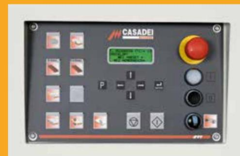
The machine is equipped with control unit placed in ergonomic position and with on/off buttons for the different working units.
