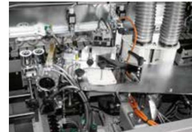
**Pre-milling unit.** The unit is equipped with 2 cutters with automatic timed intervention that ensures precise machining without damaging the panel. Anti-adhesive unit available on request.
