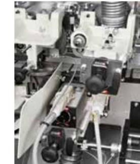
**Trimming unit.** The trimming unit is equipped with 2 high frequency motors, each one with frontal and rear pad copiers for perfect tools positioning.
